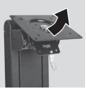
**9** Attach the bracket to the LCD panel using the four screws you removed previously.
